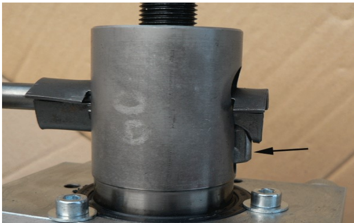
Figur 25: Make sure the sharply bent end is seated in the notch
